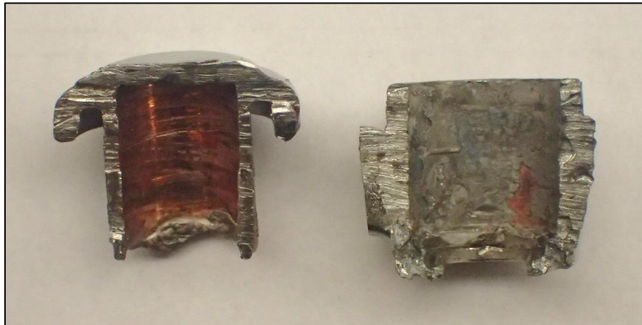
Figure 11. Teco FireBag® Device - Separated Plug from Pressed in Piece.
