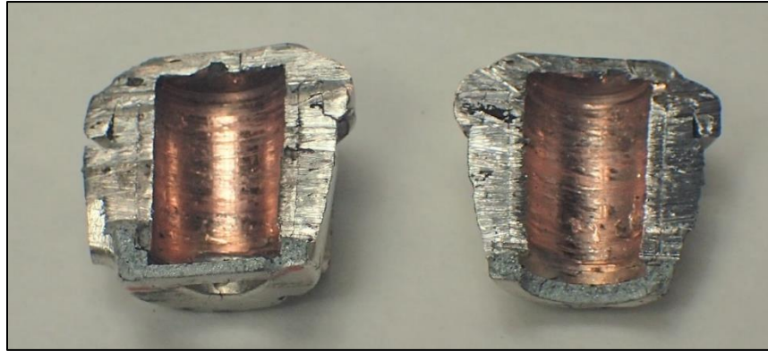
Figure 10. Teco FireBag® Device - Plug Sliced in Half.
