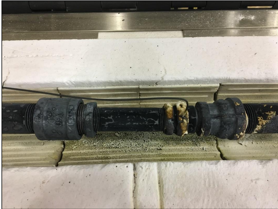
Figure 17. Teco FireBag® Device After Integrity Test.
