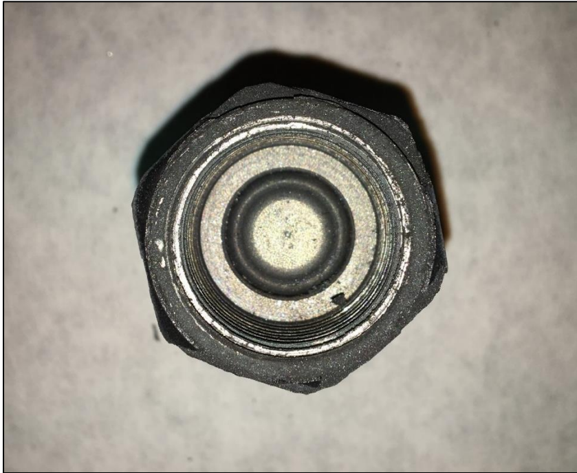
Figure 19. Teco FireBag® Device After Integrity Test - Outlet View.
